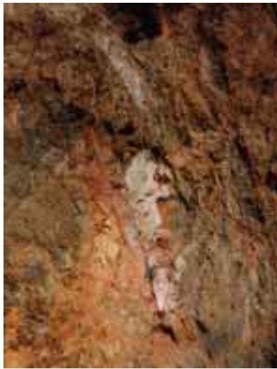
Photo.4 White to dark brown clay adhered to slate at Higashihiroshima-shi in Hiroshima Prefecture
