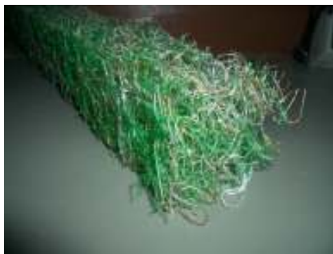
Fig.3. The modeled vegetation which is made of polyvinyl chloride
